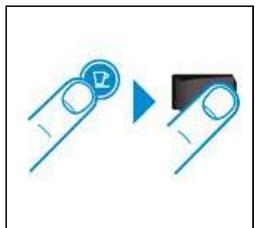
2. Press and hold Lungo button. Switch ON.
