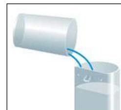
9. Refill water tank with descaling solution from container.
