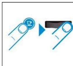
4. Press and hold espresso button, then switch on.
